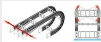
3D movements: the driver connection can be moved laterally and can be rotated by up to ± 30°
